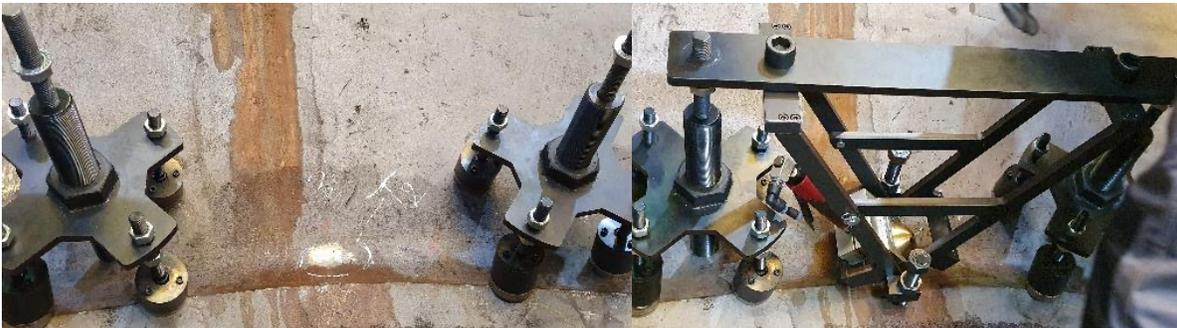
*Picture of the 8 magnet used to fix the frame (left). The frame is then set up on it to start the sampling*
